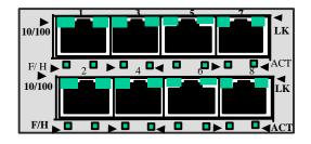
an RJ-45 port and the Link (LK) indicator for that port must be ON (indicating there is a powered-up device at the other end of the cable) in order for a LK LED to provide valid indications of operating conditions on that port.
